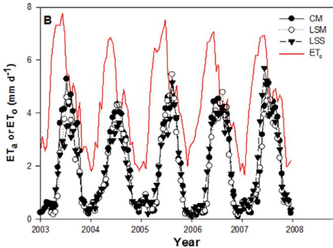
**Figure 1.** Measured ET for 2003–2007 for the three San Pedro River communities ( $ET_a$ ) vs. calculated reference ET for the sites ( $ET_o$ , red line), which approximately equals that of alfalfa. CM = Charleston mature woodland, LSM = Lewis Springs immature woodland, and LSS = Lewis Springs sacaton grassland. From Nagler *et al.* (2013).
